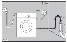
An additional drain hose and joining piece is available from your local Service Force Centre. The joining piece must have an internal diameter of 18
